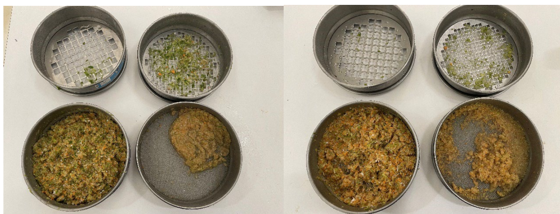
Figure 8. Left: Resulting food waste in sieves for Sample 2 (WDU-3ASAU). Right: Resulting food waste in sieves for Sample 3 (WDU-4ASAU). Note: top left sieve 13.2 mm, top right 6.7 mm, bottom left 2.36 mm and bottom right 425 \mu m.
