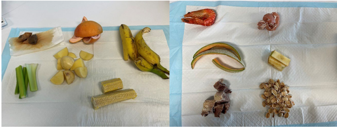
Figure 5. Left: Standard load food sample (banana peels, grapefruit rinds, celery stalks, raw potato, corn cobs, two tea bags and two paper towels). Right: Abey load food sample (prawns, egg shells, melon rinds, apple cores, meat scraps, pistachio shells).
