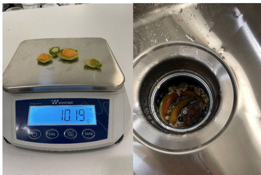
Figure 6. Left: Residual unground food waste after 3 minutes of grinding in the WDU-4ASAU device. Right: Melon rinds being pushed to the walls of the device chamber.
