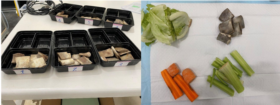
Figure 7. Left: Example of rib bones load food samples for bone grinding rate test. Right: Mixed load food sample for the degree of fineness test.
