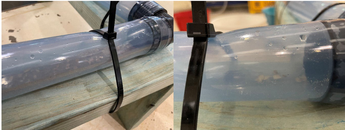
Figure 9. Left: Rib bone and pistachio shell particles remaining on the 90-degree bend after grinding. Right: Rib bone and pistachio shell particles remaining on the 90-degree bend after 5 flushes.
