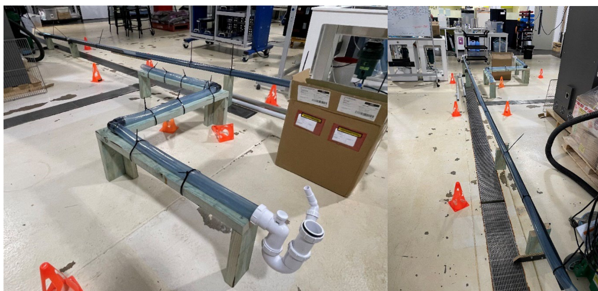
Figure 4. Left, 3 m long pipe setup with 2 bends (DN 50). Right, 6 m long straight pipe setup (DN 50).
